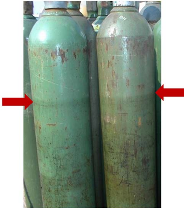
Figure 1—Example of cylinders with a water line
